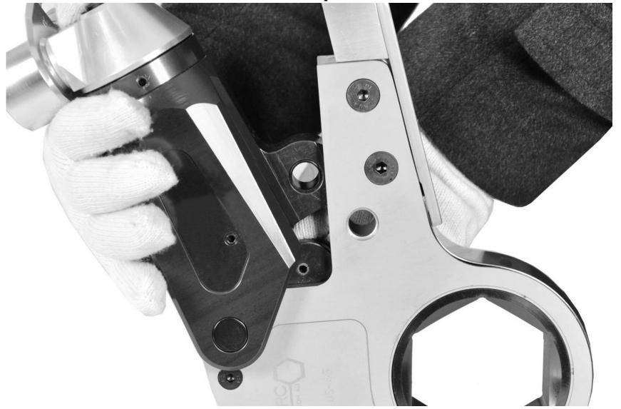
Do not stop stressing the drive plate until it is almost on the same plane with the side plate
